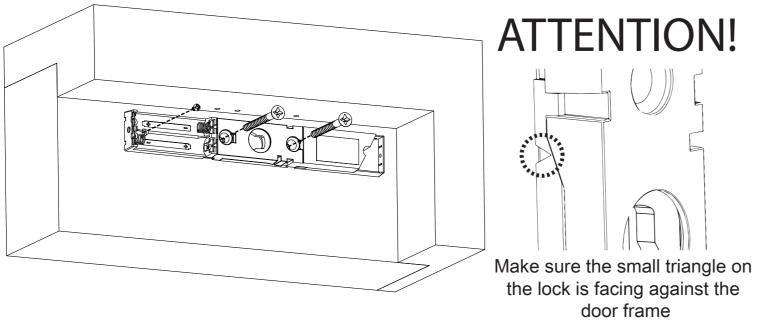
Open the door and mount the angle bracket on the door frame
